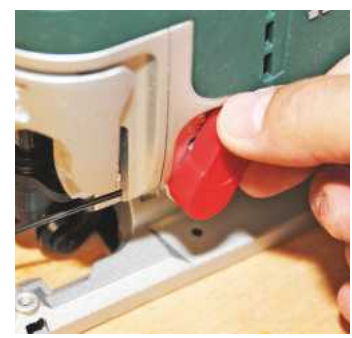
▲ The lever for the pendulum action looks a little cheap but works perfectly
